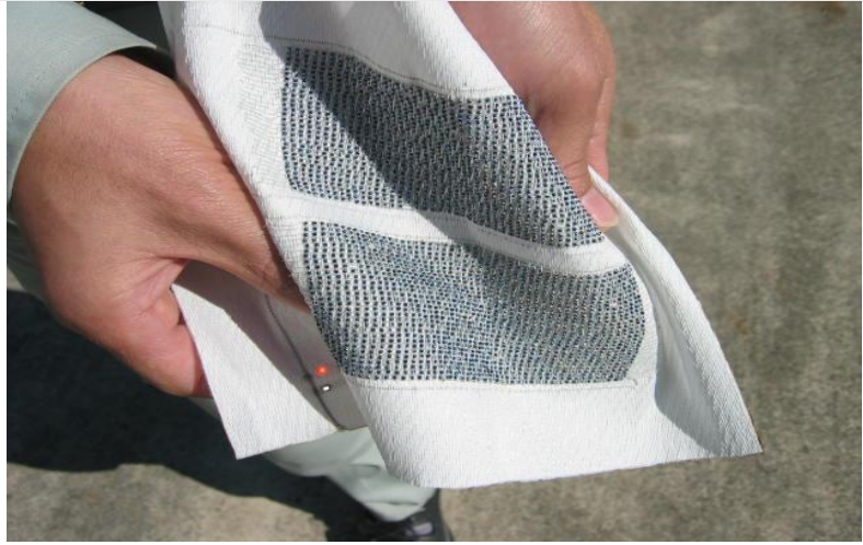
Light, thin and flexible photovoltaic textiles woven using photovoltaic yarn
